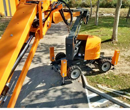
These 4x4 Boom Lifts from ATN are extremely unique in the fact they can be used as a conventional self-propelled Boom Lift, alternatively the jacks (stabiliser legs) can be deployed from the basket to level the machine on uneven ground. Brilliant? Too right!
